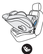
LATCH: Lower Anchor Belt DO NOT install by this method for a child weighing more than 35 lbs (15.9 kg).
