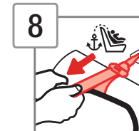
7 Tighten Belt Place hand in child restraint. Firmly push down while pulling free end of belt to tighten.
