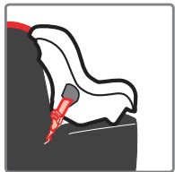
Lower Anchor Belt with Tether
